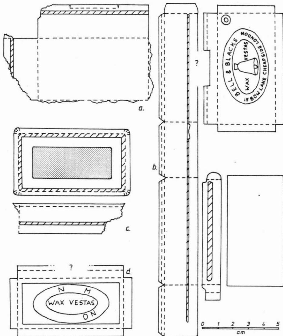
FIGURE 5. Matchboxes: a. all in one base; b. Bell and Blacks variety; c. Belgian Mars; d. Bryant and May.
