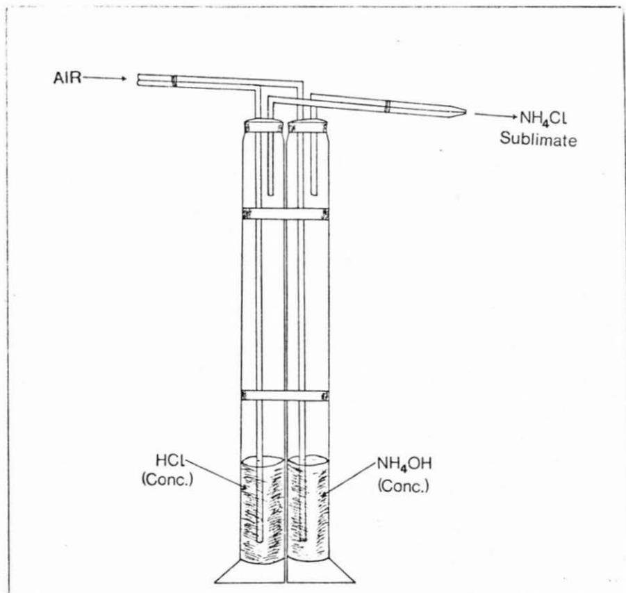
FIGURE 1. Apparatus for coating obsidian tools so as to enhance their photographic perspective (from Bassler, 1953:G20).
