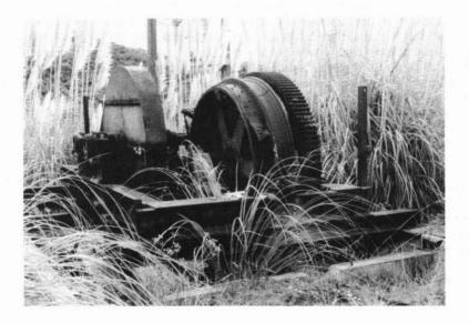
Plate 2. Winding gear and motor, Rotowaro No. 1 mine (S14/149).
