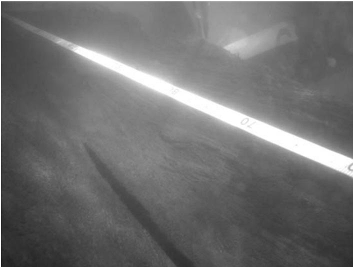
*Figure 5. Hull section near 'prow' showing split near keel (photo Diver Services Ltd.).*
