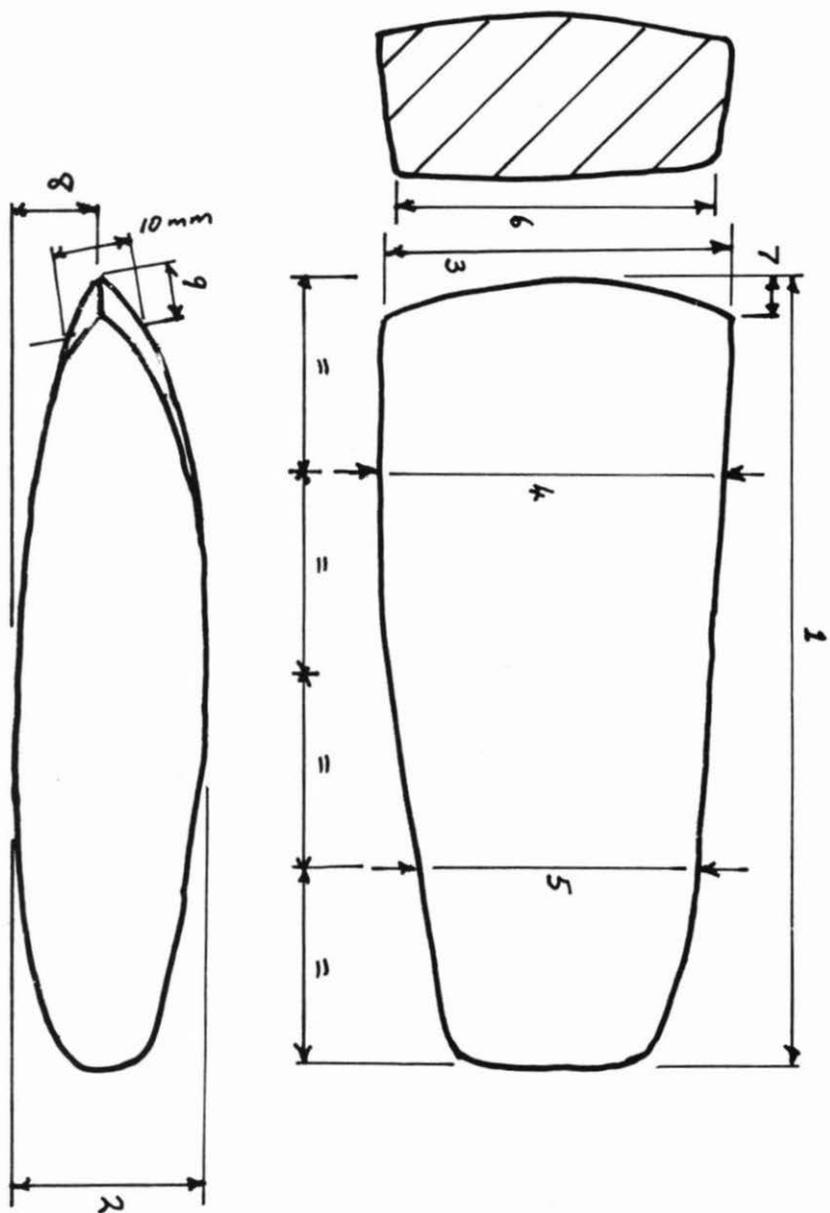
Figure 1. Dimensions recorded defining the shape of the adzes. Dimensions 4 and 5 are on the face of the adze. Dimension 6 is on the back at 1/4 length.
