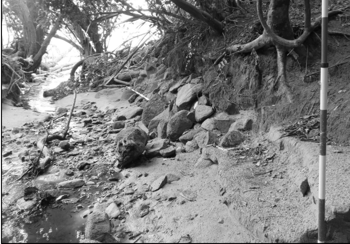
Figure 5. Looking towards the mouth of Hydro Creek: the sand deposited and scoured between Jan– Sept 2019, after the installation of site protection for the eastern bank (true right), D48/5 Area 1 (Photo: Brooke Tucker).
