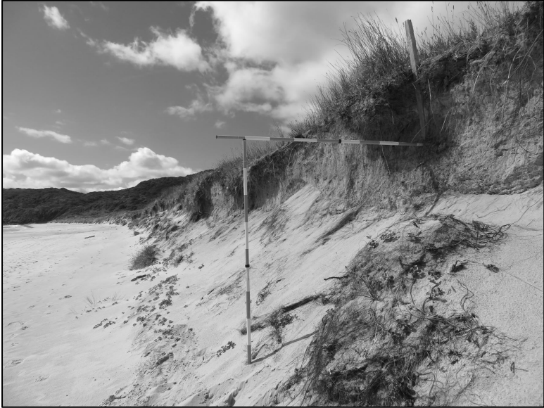
Figure 4. Monitoring dune movement with reference to eroding marram grass survey pegs. Sealers Bay, Whenua Hou, January 2019 (Photo: Brooke Tucker).
