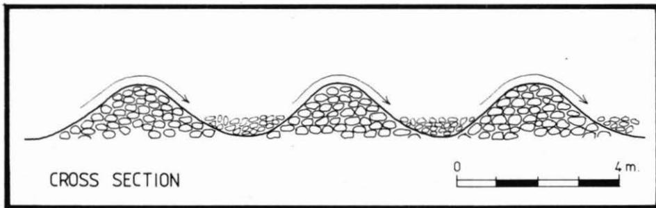
Figure 8: Cross section showing backfilling between tailings rows.
