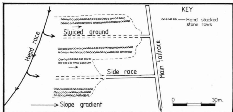
Figure 4: Diagram of blow down system of sluicing adapted from Park (1908:48).
