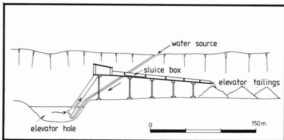
Figure 17: Simplified diagram of a hydraulic elevator in operation.
