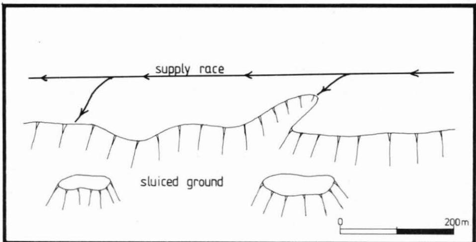
Figure 16: Diagram of a sluice face.
