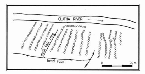
Figure 7: Diagram of S124/115 parallel tailings, Sandy Point, Upper Clutha River. For key, see Fig. 4.
