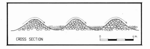
Figure 8: Cross section showing backfilling between tailings rows.
