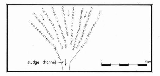
Figure 12: Diagram of a fan tailings site, S124 / 105, Luggate area. For key, see Fig. 4.
