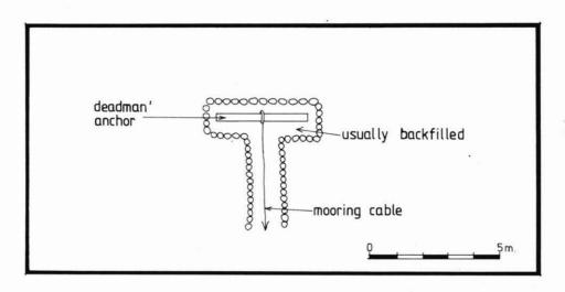
Figure 19: Dredge mooring anchorage.
