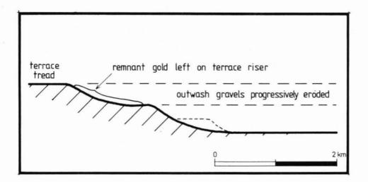
Figure 5: Cross section of terrace scarps showing locatin of blow down tailings.
