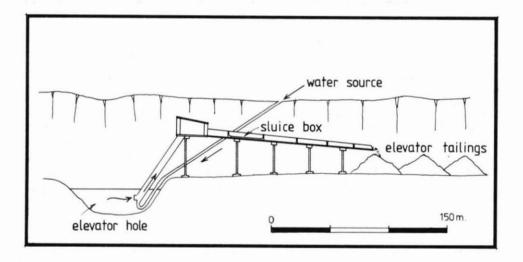
Figure 17: Simplified diagram of an hydraulic elevator in operation.
