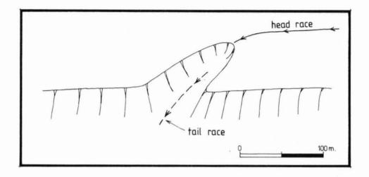
Figure 15: A sluicing scar site.
