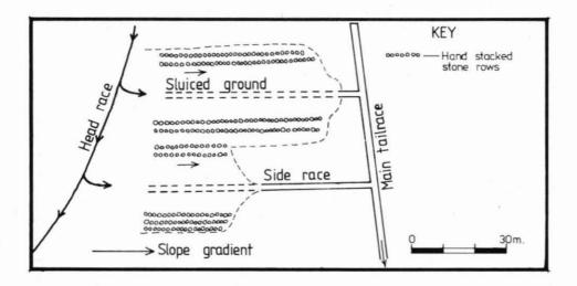
Figure 4: Diagram of blow down system of sluicing adapted from Park (1908:48).
