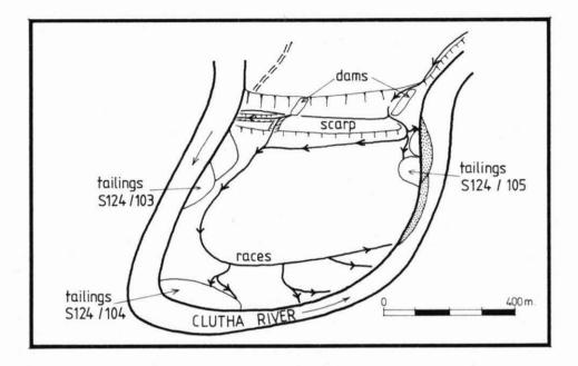
Figure 13: An interrelated races, dams and tailings system, near Luggate.
