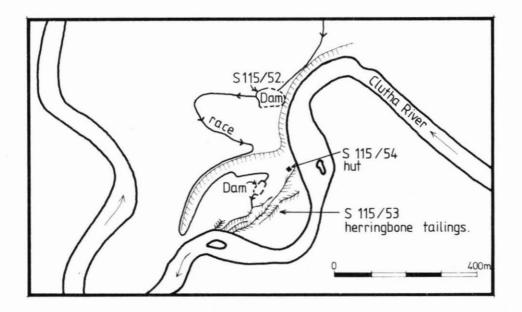
Figure 3: Diagram of herringbone workings (Site S115/53) Ah Wee's Point, Clutha River, within dams, races, and tailings complex (Sites S115/52–54).
