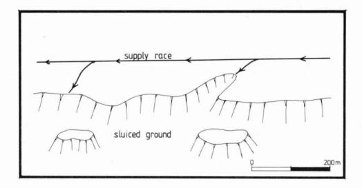
Figure 16: Diagram of a sluice face.
