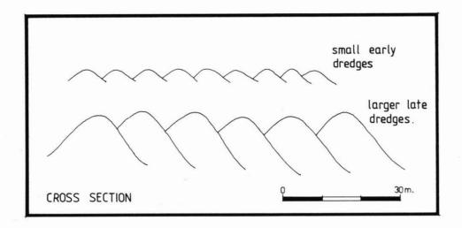
Figure 18: Diagram of dredge tailings in cross section.
