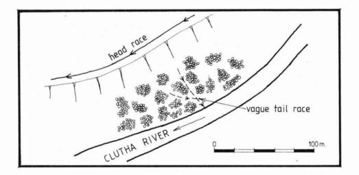
Figure 14: Diagram of an amorphous tailings site in the Luggate area showing typical hummocky mounds.
