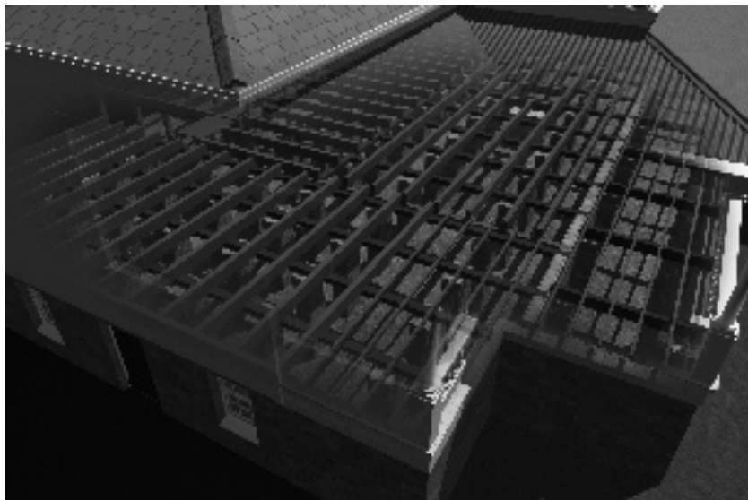
Figure 7. View from NE corner of the house showing floor joists and beams.
