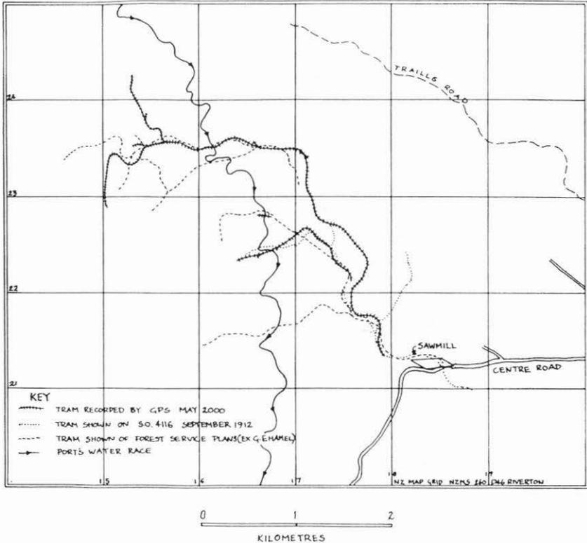
Figure 3. Overlay of GPS survey of Buchanan's Tram with contemporary plans of tram line.
