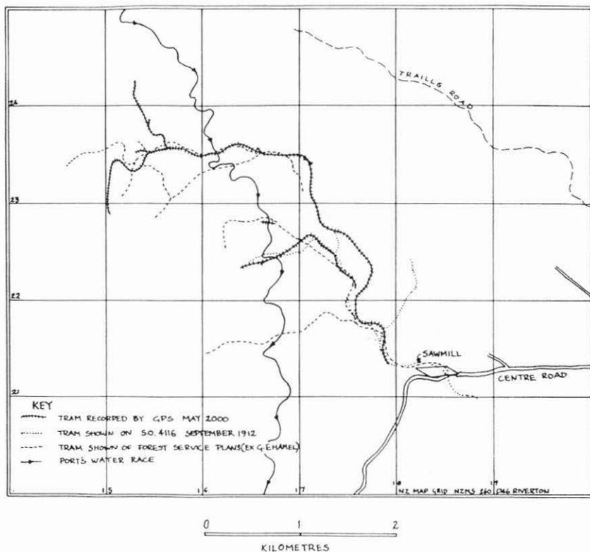
Figure 3. Overlay of GPS survey of Buchanan's Tram with contemporary plans of tram line.
