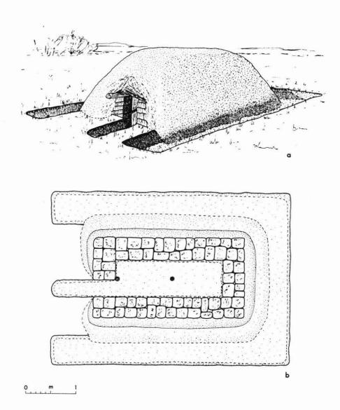
FIGURE 2. Perspective view and plan of finished kumara storage pit.
