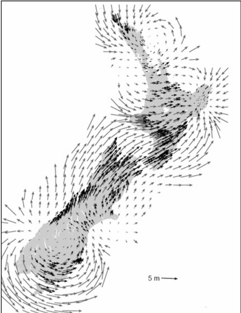
*Figure 1. This shows the differences between NZGD1949 and NZGD2000 after applying the 7 parameter similarity transformation (Land Information New Zealand 2010d).*
