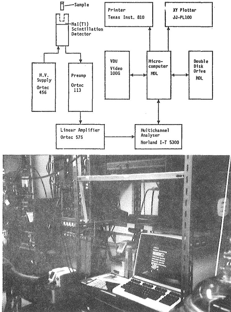
Figure 4: Block diagram of the gamma-ray spectrometer (above); photograph of the same (below).
