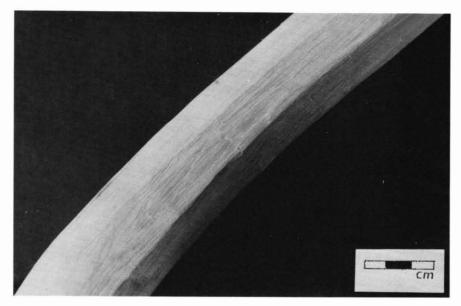
Plate 5. Shaping hardwood using a high angle scraper.
