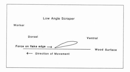
Figure 2. Force exerted on scrapers during the working of hardwood. Note the angle of the flakes when used in relation to the position of the worker. High angle scrapers are pulled towards the worker, whereas the low angle scrapers are pushed.
