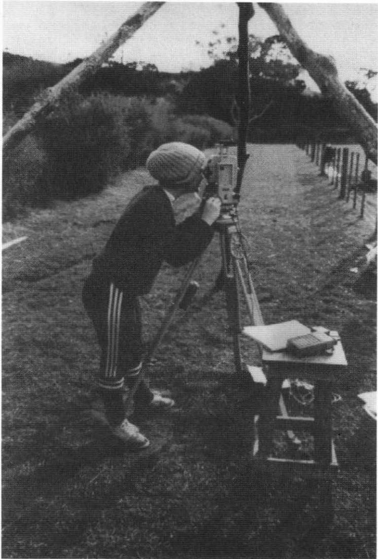
Plate 2. The theodolite set up over the site datum during the excavation of S11/20. One of the students is focusing the theodolite while the data logger rests on the stool.
