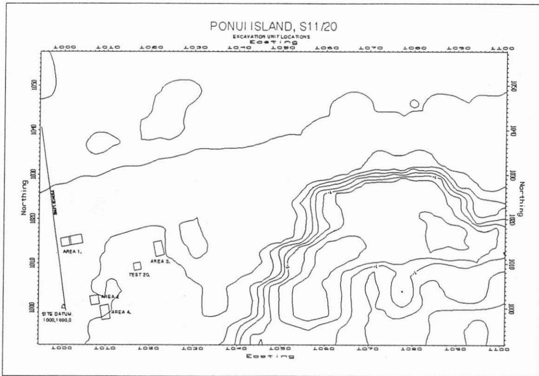
Figure 1. A topographic plan of S11/20 showing the location of the major excavation areas and the site datum. This plan was generated in the field using data obtained with the theodolite.
