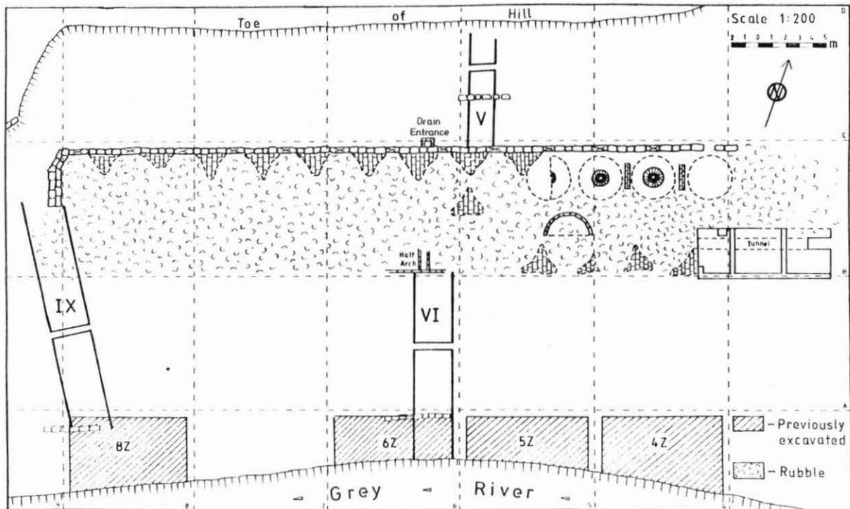
FIGURE 1. Brunner coke ovens excavation plan.
