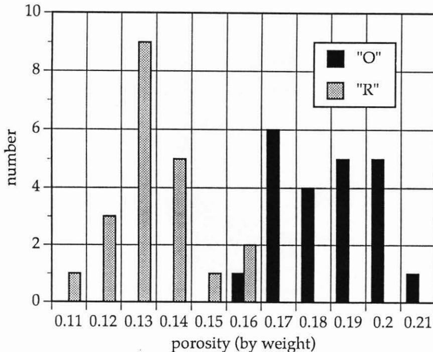
Figure 7: Histogram of porosity by weight for classes 'O' and 'R' bricks.
