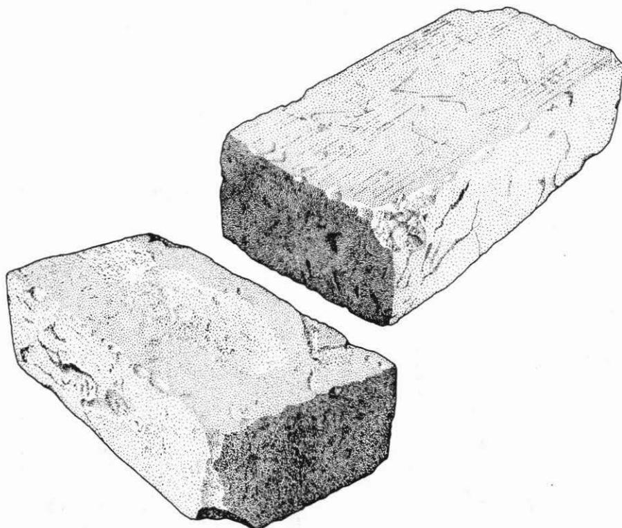
Figure 6: A typical brick from the furnace. Top: upper, or strike, face showing strike marks. Bottom: lower, or stock, face showing indistinct frog. Dimensions approximately 220 x 100 x 70 mm.
