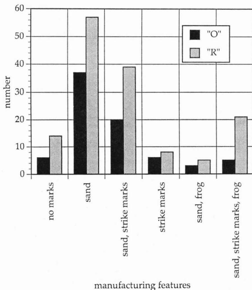
Figure 9: Manufacturing marks in 'O' and 'R' class bricks.
