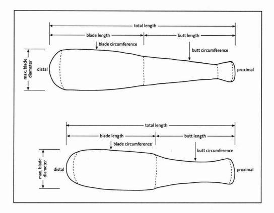
Figure 3: Key measurements taken on beaters/pounders.
