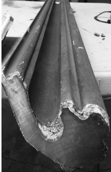
Figure 20. Kauri scotia or cornice moulding probably made with several different cutters, c.1890.
