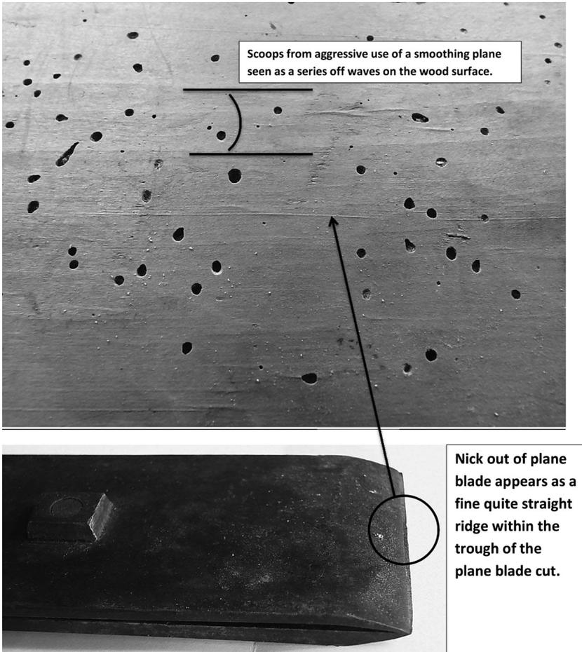
*Figure 8. Smoothing plans marks evident as slight waves on the timber surface. Nicks in the blade create thin ridged lines.*
