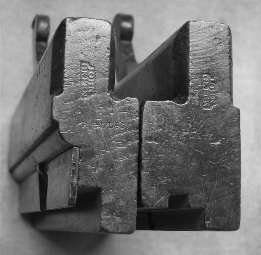
*Figure 10. A matched pair of tongue and groove planes by John Green, London, c.1780.*
