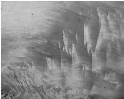
*Figure 5. Compression grain in tōtara.*
