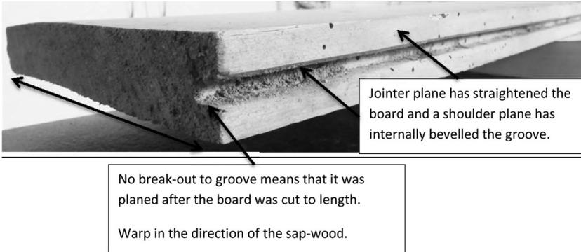
*Figure 12. Hand saw marks to the board end but no break-out in the groove indicate that planing occurred after cutting.*
