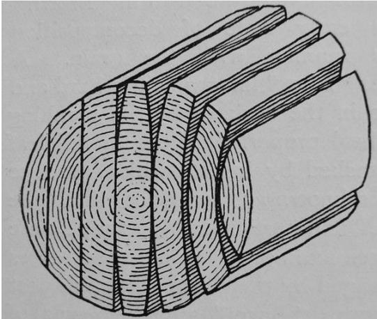
*Figure 4. Distortion patterns for quarter and cross-cut timber.*
