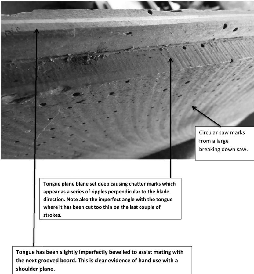
*Figure 11. Chatter marks clearly indicate a hand-planed tongue.*
