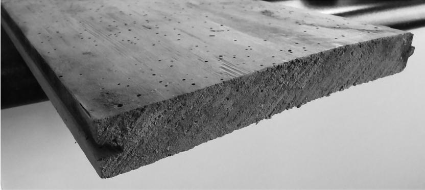
*Figure 3. Contamination to the planed top surface of the kahikatea board and cupping towards the underside.*
