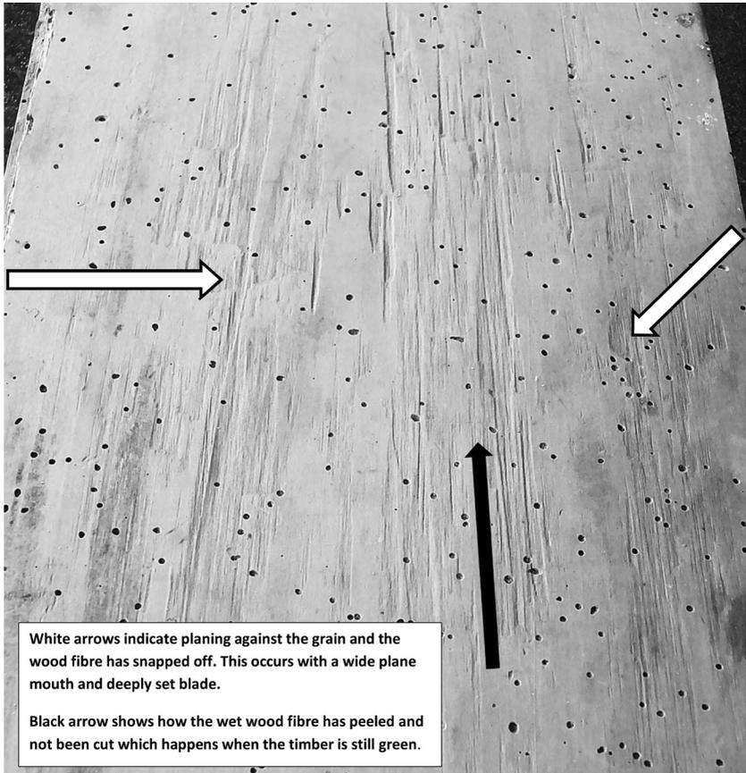
*Figure 9. Break-outs caused by the plane's blade being set too deep. Tear marks indicate that the wood was planed too soon after the tree was felled.*
