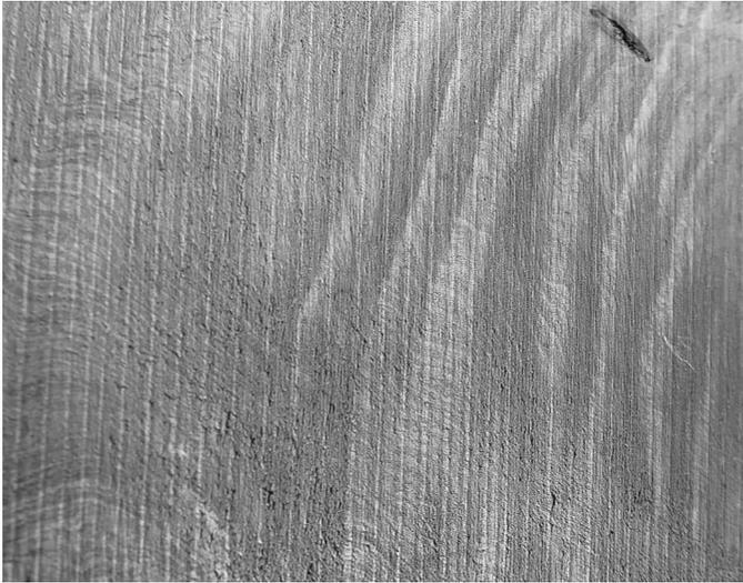
*Figure 17. The parallel lines are caused by the weld or join in altering the band-saw blade tension. Each line represents one full revolution. Compression grain to a piece of Southland beech.*
