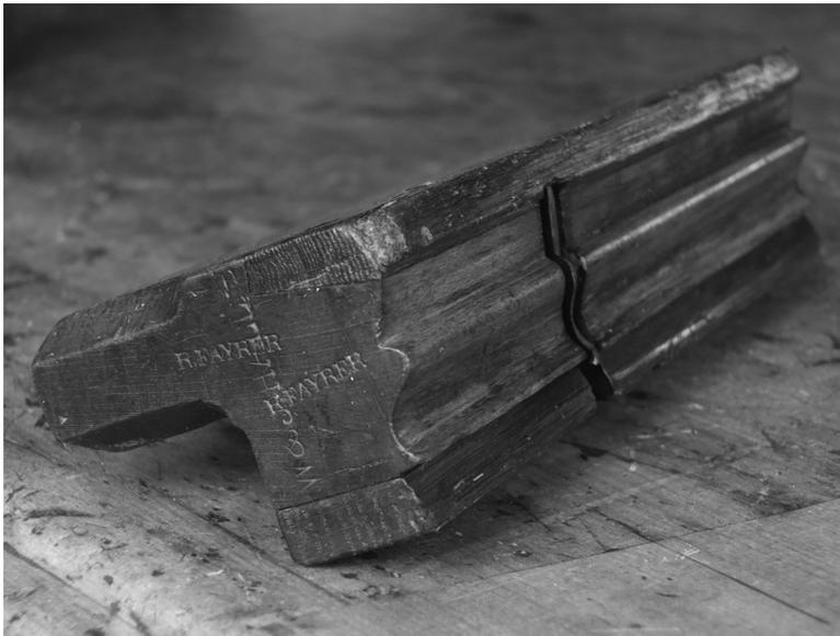
*Figure 13. Grecian ogee moulding plane sole, c.1820.*
