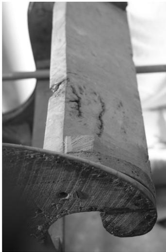
*Figure 16. The saw marks on the back of the sofa.*
