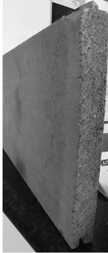
*Figure 6. Break-outs can be seen on the underside of the board, as well as cupping and a light band of reduced photo-oxidation.*
