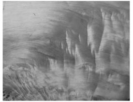
Figure 5. Compression grain in totara.
