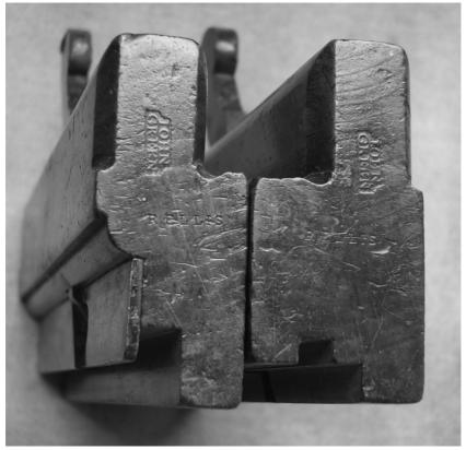
*Figure 10. A matched pair of tongue and groove planes by John Green, London, c.1780.*
