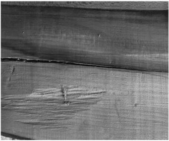
*Figure 19. Fine ripples on this piece of birch indicate mechanical planing. The rough area at bottom left is from a chainsaw.*
