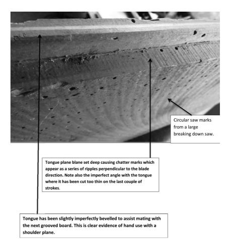
Figure 11. Chatter marks clearly indicate a hand-planed tongue.
