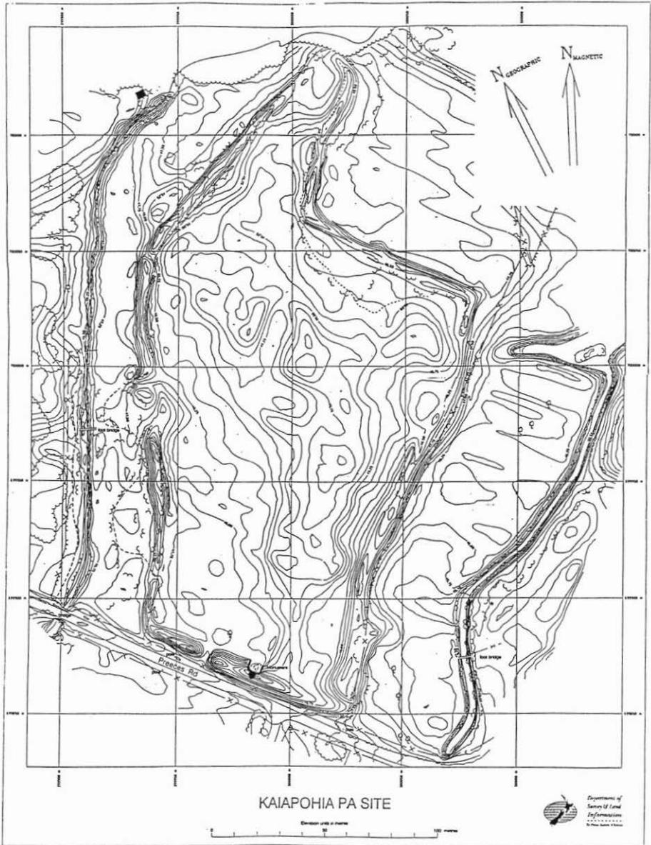
Figure 2. Contours of elevation from the digital terrain model at the Kaiapohia Pa site measured by photogrammetry. Contour interval 0.25 m.
