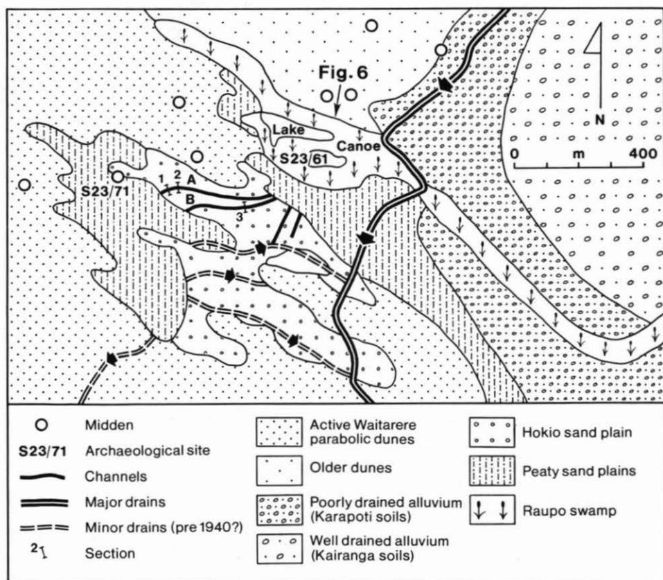
Figure 2: Te Awamate lagoon, associated soils, and the location of channels, based in part on Campbell (1979), Bailey and Kozyniak (1984), and aerial photographs. Section numbers refer to Figure 6.
