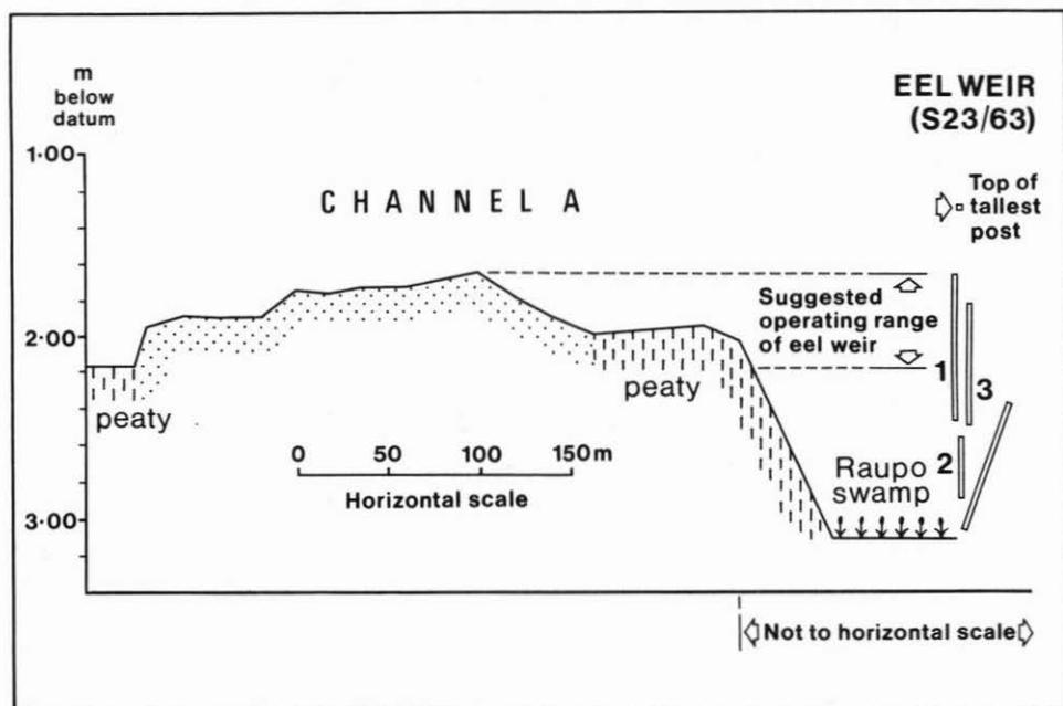
Figure 5: Levels along the length of channel A; levels of eel weir (S23/63) are reduced to the same datum. The positions of the posts numbered 1 to 3 are shown on Figure 6.
