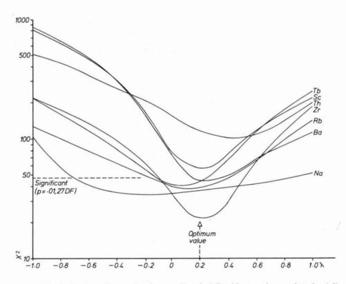
Figure 5: Bartlett's  $\chi^2$  test for equal variance uniformly fails with trace element data ( $\lambda = 1.0$ ); however, a power transformation of the form  $x' = (x^{\lambda} - 1)/\lambda, \lambda \neq 0$ ;  $x' = \log_e x, \lambda = 0$  results in a dramatic improvement, especially with  $\lambda \approx 0.2$ . This figure illustrates the effects of the transformation for a selection of elements for New Zealand and Oceanic obsidians.
