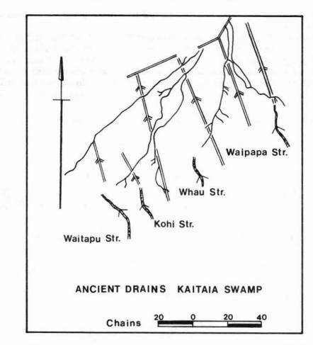
Figure 8: Ditch system in wetlands at Pukepoto, Kaitaia catchment. Category D. Redrawn from Wilson 1921. For identification of map symbols, see key at Figure 2.
