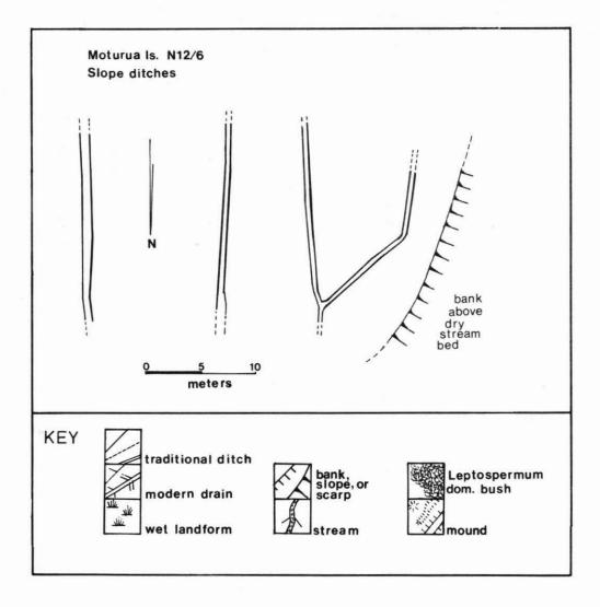
Figure 2: Ditch system N12/6, Moturua slope garden, Bay of Islands. Category A. Redrawn from Peters 1975. Slope gradient is approximately 20°. Key also applies to Figures 3 and 6-10.
