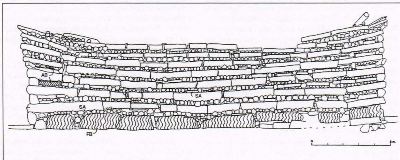
FIGURE 4.5. Face view of columnar lava construction in the southwest side of the main entry wall, Nan Douwas tomb, Nan Madol. Rock type codes are the same as in Figure 4.6.
