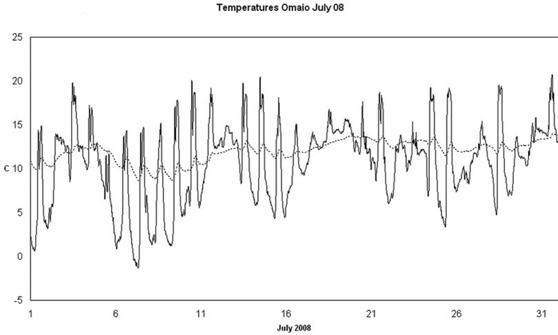
Figure 1. July 2008 external temperature (black line) and internal rua temperature (dashed line) at Omaio.
