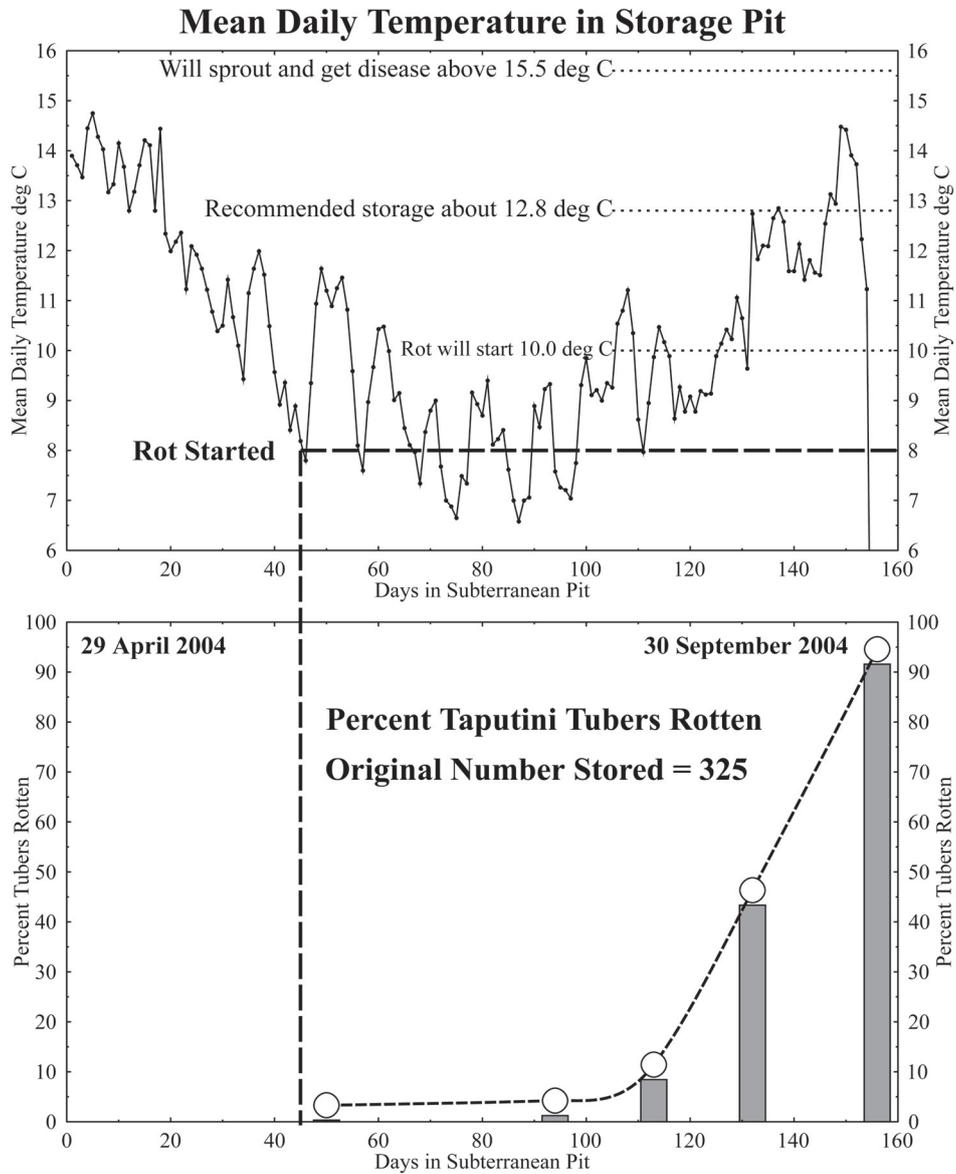
Figure 15: The mean daily air temperature inside the pit over the entire period of storage, together with the percent of tubers found to be rotten. See text.
