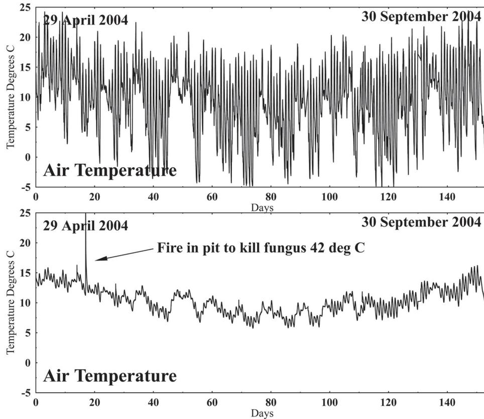
Figure 13: Air temperature records for the entire 154 day period of storage. Upper: the control station. Lower: inside the pit. See text.
