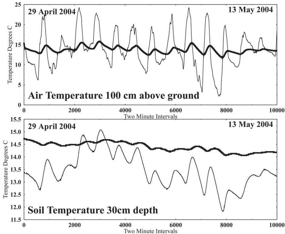
*Figure 12:* Diurnal changes and temperature lag in the experimental storage pit and control. The bold lines relate to the experimental storage pit and the fine lines to the control station. The air temperature loggers were 100 cm above the floor of the pit and inside the control station 100 cm above the ground surface. The soil temperature probes were 30 cm beneath the pit floor and 30 cm beneath the ground surface under the control station.
