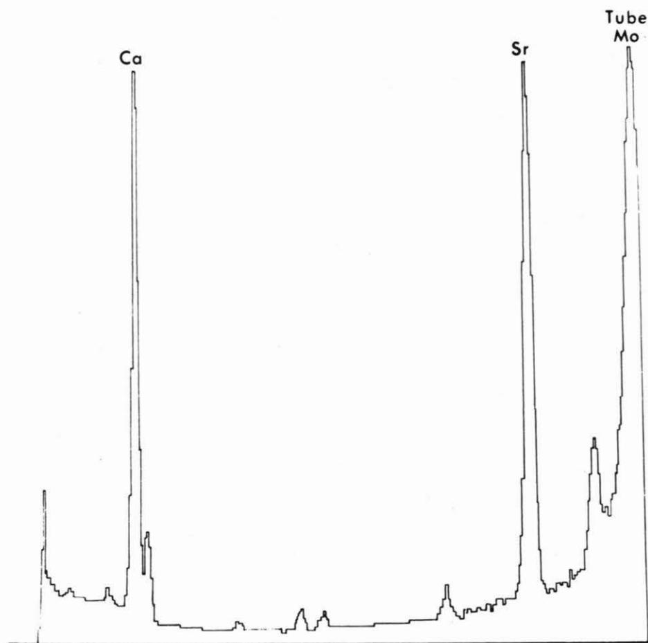
Figure 3 X-Ray Fluorescence Spectrum of one of the small ivory reel units. Note the very large strontium peak which is distinctive of *Dugong dugon*.
