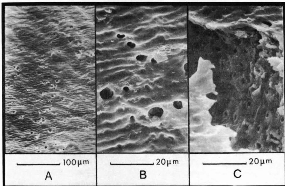
Figure 2 Scanning electron micrographs of one of the small ivory reel units. A: x 200, B: x 1000, C: x 1000. Note the surface rippling in A and B and the lateral interconnecting canaliculi in C.
