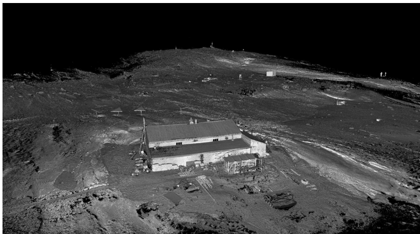
Figure 6. Terra Nova hut and local environs consisting of sixty point clouds registered together.
