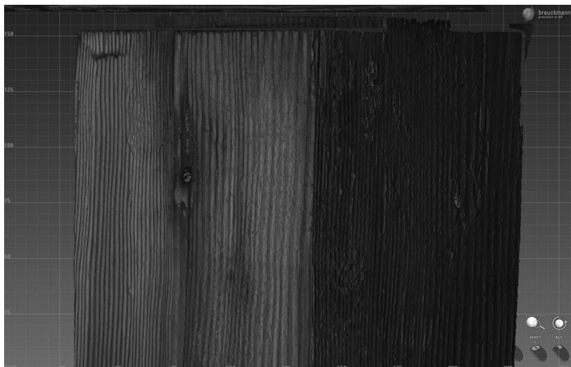
Figure 5. Section of ablated surface from a veranda post, main entrance of Discovery Hut.
