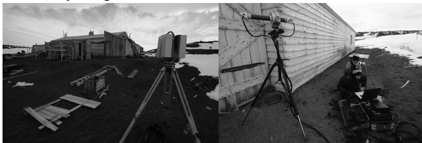
Figure 2. Exterior scanning using the Leica 6100 (left) and the Breuckmann3D-HE (right) at Terra Nova Hut.
